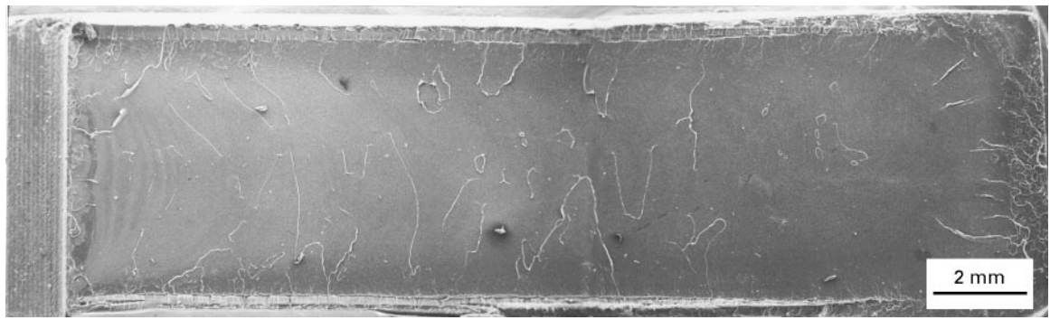
Figure 7 Fracture surface of a notched PS sample broken in a slow strain-rate test with edge-on UV exposure following 5 weeks edge-on UV pre-exposure.
